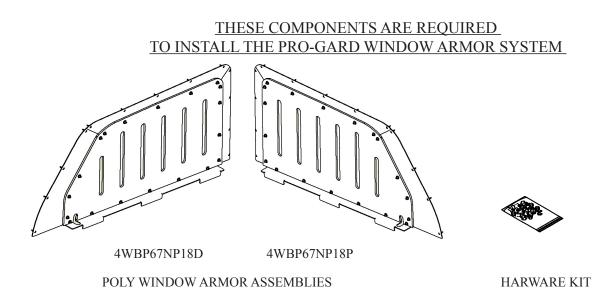
THIS WINDOW BARRIER IS ONLY USED WITH THE OEM DOOR PANEL.
