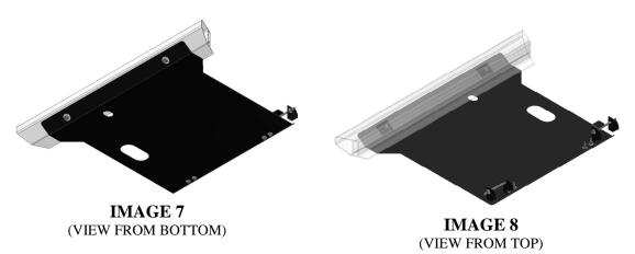
III. When all hardware is attached and the skid plate is installed correctly, go back and tighten all bolts.
