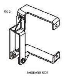
B. Repeat procedure for the driver's side. Place a small level on top of brackets once leveled **tighten all fasteners**.
