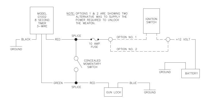
B. Connect the gun lock wiring as shown in the diagram above.
