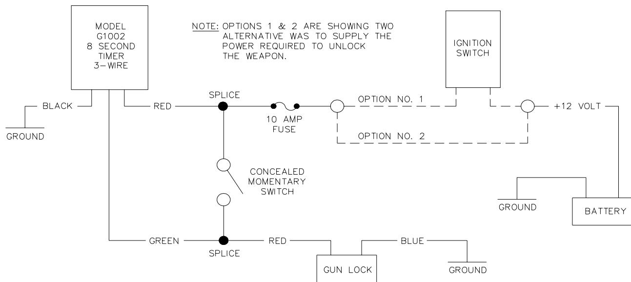
Note: If for any reason the gun lock momentary switch remains activated, such as, the button is damaged, and/or shorted, the unit will time out in 8 seconds and can not be operated again until the defective switch is repaired, thus saving the gun lock solenoid. Do not connect directly to power for more than 20 seconds!
