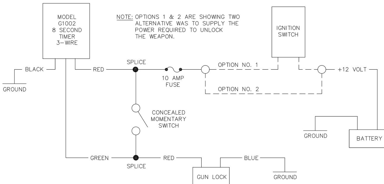
**NOTE:** *Pro-gard requires the use of a 10 AMP fuse between the power source and gun lock circuit or the warranty will be voided!*
