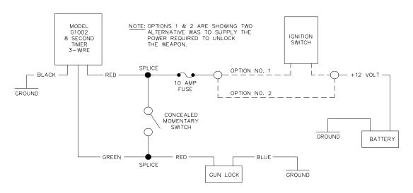
If for any reason the gun lock momentary switch remains activated, such as, the button is damaged, and/or shorted, the unit will time out in 8 seconds and can not be operated again until the defective switch is repaired, thus saving the gun lock solenoid. Doot connect directly to power for more than 20 seconds!
