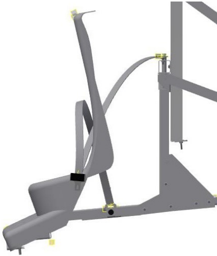
C. Place the seat loosely inside the vehicle. Pass the seat belt through the (3S5003) seat belt bezels, then through the rectangular holes in the middle of the seat.
