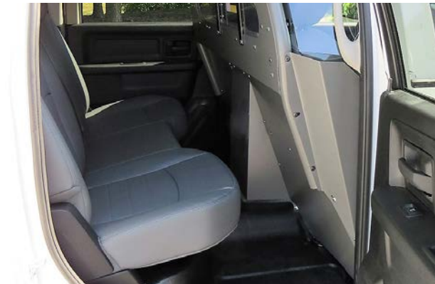
Space Saver Partition shown in the 2015 Dodge Ram SSV Truck
