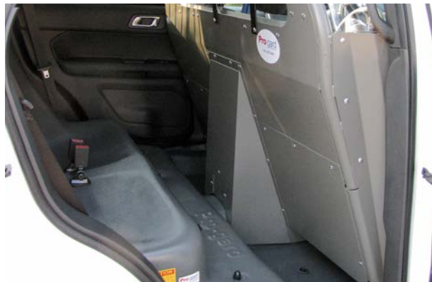
Space Saver Partition shown in the 2013 Ford Police Utility Interceptor
